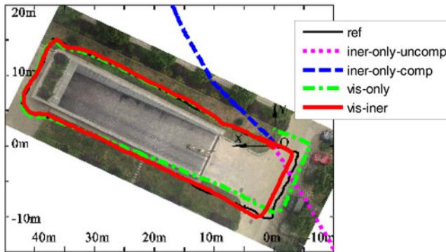
Figure 4. Estimated path in the horizontal plane for iner-only-uncomp (sensor biases ignored), iner-only-comp (sensor biases compensated), vis-only and vis-iner solution. The iner-only-uncomp and iner-only-comp solutions exceed the scale of the map after 70 and 76 seconds, respectively. The path estimated by vis-iner agrees well with the known path (the black line) and shows smaller errors in position and heading than the vis-only solution.
