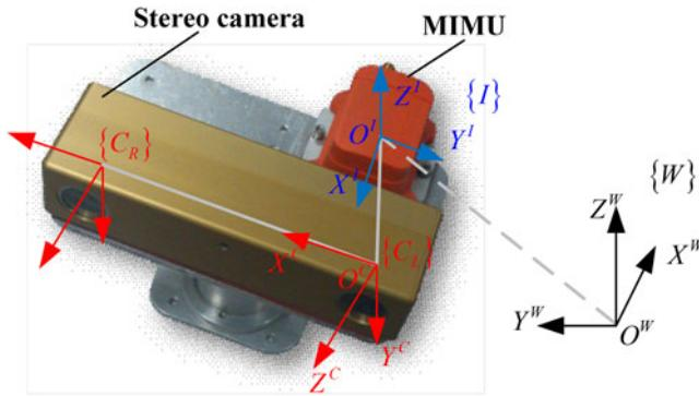
Figure 1. The VIS which consists of the stereo camera and the MIMU and the relationship between the world  $\{W\}$ , camera  $\{C_L\}$ ,  $\{C_R\}$ , and IMU  $\{I\}$  reference frames. The stereo camera and the MIMU are rigidly attached.
