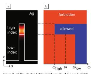
Figure 2. (a) The electric field intensity profile of the excited SPP mode within the SPP cavity. (b) The band diagram for the SPP mode corresponding to (a) shows allowed and forbidden regions drawn along the z-axis.
