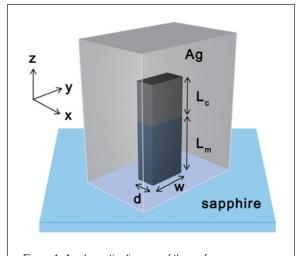
Figure 1. A schematic diagram of the surface plasmon polariton (SPP) cavity—a silver-covered dielectric nanorod consisting of a high-index material (dark grey) on top of a low index material (blue)—placed on a sapphire substrate.
