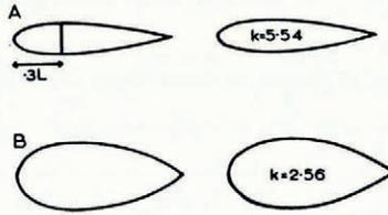
Fig. 1. (a) Standard aircraft wing profile, without camber. (b) Section of a U.S. Navy No. 1 Strut (after Von Mises). Approximating lemniscate loops, together with the values of  $k$ , appear throughout
