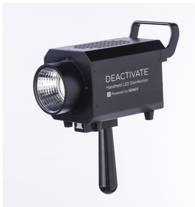
Figure 2. Handheld ultraviolet light-emitting diode device used for this study.
