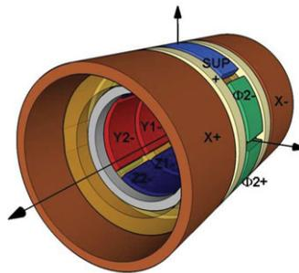
**Figure 3.** Electrode configuration : the electrode pairs, etched on gold-coated silica cylinders, control the six degrees of freedom of the engaged test-mass.
