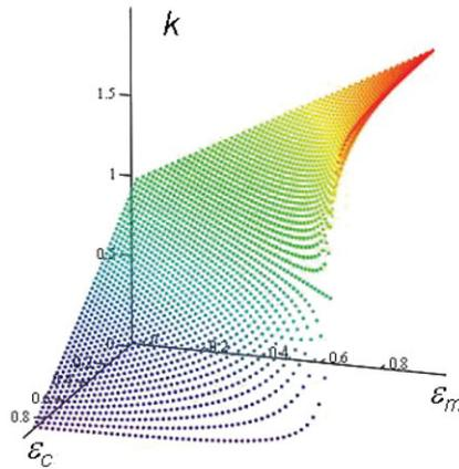
**Figure 4.** Correction factor of the radiation pressure model, function of the mass and cage reflectivities.
