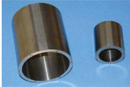
**Figure 2.** Test-masses featuring flat panels for axial rotation control and holes for displacement limitation.
