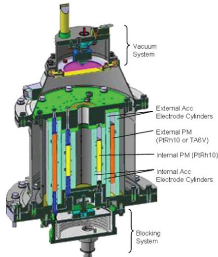
**Figure 1.** Cross cut view of the differential accelerometer, consisting of the sensor core of test-masses and electrode cylinders, the blocking mechanism below and the vacuum system above.
