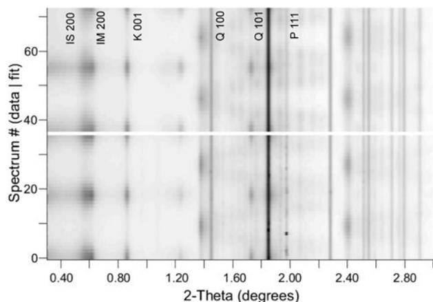
Figure 3. Stack of diffraction patterns for Kimmeridge shale,  $\varphi=0^\circ$  tilt image. Experimental data at bottom and Rietveld fit on top. Some diffraction for lines for illite-smectite (IS), illite-mica (IM), kaolinite (K), quartz (Q) and pyrite (P) are labeled.
