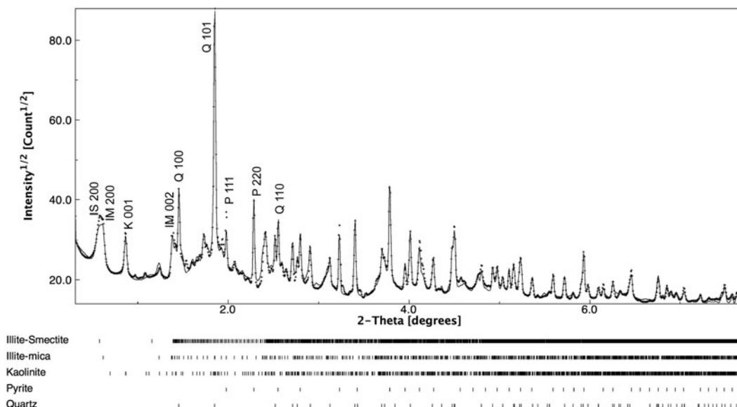
Figure 6. Cumulative plot for all patterns of the  $\varphi = 0$  image at the end of refinement cycles with seven images, full  $2\theta$  range. Dots are experimental data and line is Rietveld fit. Some diffraction peaks are labeled (IS, illite/smectite; IM, illite/muscovite; Q, quartz; P, pyrite).
