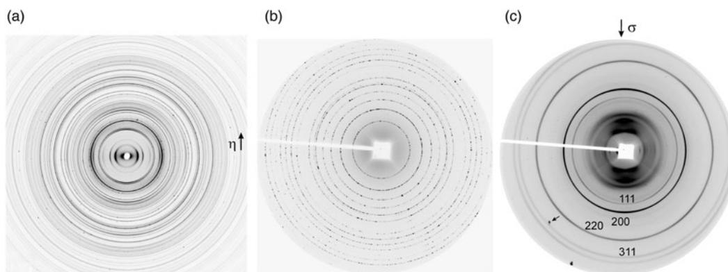
Figure 2. 2D synchrotron diffraction images. (a) Kimmeridge shale with many phases, some with strong preferred orientation. (b)  $\text{LaB}_6$  standard used for the DAC experiment, rather coarse-grained and with some impurities. (c) Radial diffraction DAC experiment on ferropericlasite. Arrow points to a diffraction spot from diamond. The compression direction is vertical.
