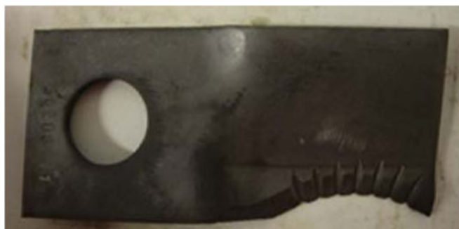
Figure 12. Serrated blade design with strip-shaped serrations (Gan et al. 2018).
