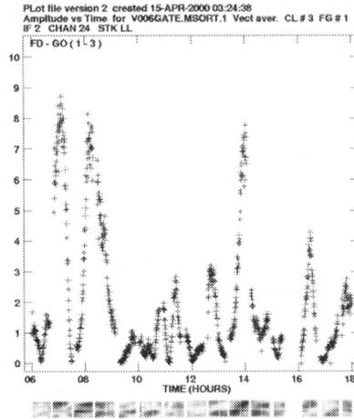
*Figure 1.* Visibility amplitude vs time for the Fort Davis – Green Bank baseline. Data for Ch 24 of IF2 is shown above the corresponding dynamic spectrum. The lower frequency channels lie at the bottom, higher frequencies correspond to higher levels in the dynamic spectrum bar; the bar width is  $\sim 32$  MHz. The darker areas correspond to higher visibility amplitude. The same dynamic spectrum is shown on Figure 2.
