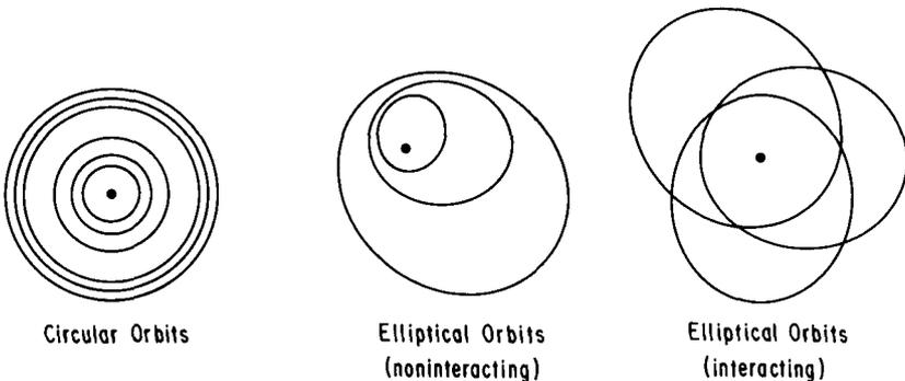
Figure 2.—Particles in circular orbits (or in nonintersecting orbits with  $\epsilon \neq 0$ ) experience no collisions. Collisional evolution only occurs when these elliptical orbits intersect. Kepler orbit:  $\Phi(r) = -k/r$ .
