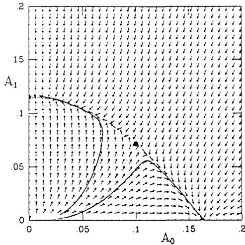
Fig. 2. Flow field for nonresonant two-mode case; Separatrices: *thin lines*; Evolution of hydro-model: *thick lines*.
