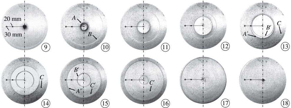
FIGURE 7. Sequence of schlieren images showing the propagation of shock waves in observation region for  $Ma_0 = 1.17$ , which is a continuation of figure 5. Again, the frame rate of the high-speed video camera is 105 000 f.p.s. corresponding to a time interval between two consecutive frames of about  $9.52 \mu\text{s}$ . The number in the lower right corner of each image represents the sequence of the images. The locations of 20 and 30 mm away from the focal point are marked.
