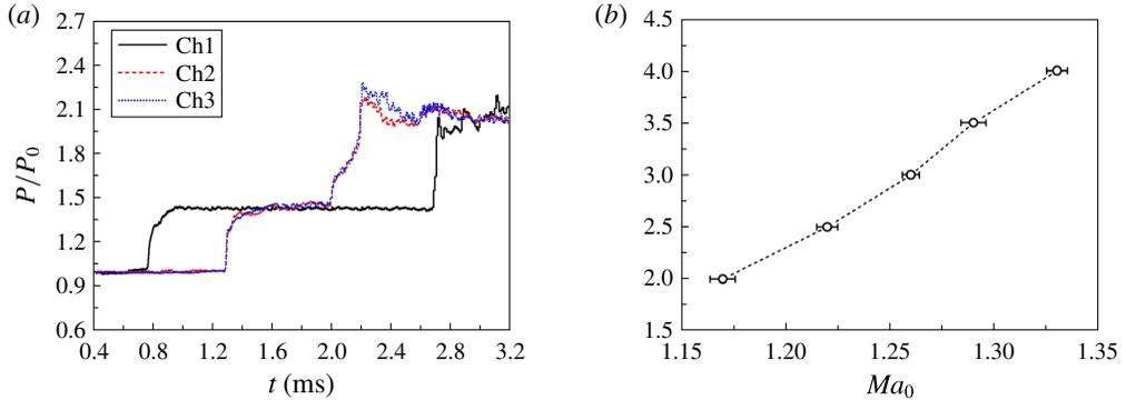
FIGURE 4. (Colour online) (a) Pressure histories of transducers Ch1–Ch3 mounted on the sidewall of the driven section for  $Ma_0 = 1.17$ . (b) Experimental measurements showing the pressure ratio between the driver and the driven sections versus the value of  $Ma_0$ .
