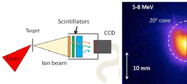
**Figure 8.** (Left) Schematic for a three-color proton beam spatial profiler. Higher-energy protons are stopped in the shorter-wavelength scintillators located further downstream in the stack. The combined optical signal is collected and relayed to a CCD camera via a fiber optic bundle. (Right) Proton (half) beam profile for a 100 nm Al target irradiated at  $5 \times 10^{20}$  W/cm<sup>2</sup> with high contrast ( $>10^9$ ).
