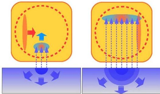
**Figure 15.** Electro-optical encoding. (Left) EO crystal (yellow square) acquires a local birefringence when the electric field (dashed arrows) reaches it. (Right) The probe laser, starting with a well-defined linear polarization, crosses the crystal while the charge propagates on target, increasing the source size<sup>[31]</sup>.
