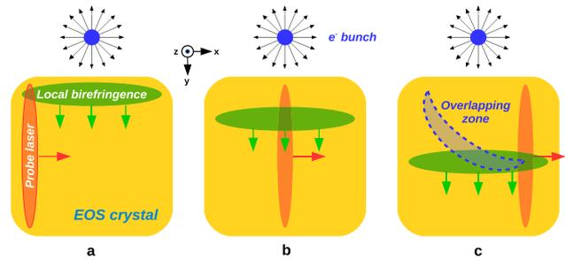
**Figure 13.** Spatial encoding process: (a) the coulomb field, relative to the electron bunch, makes the crystal birefringent; (b) while the E-field propagates into the crystal, the local birefringence shifts downwards; (c) the probe laser crosses the crystal and its polarization is rotated: the resulting signal comes from the region where the local birefringence and the probe laser are temporally overlapped<sup>[29]</sup>.
