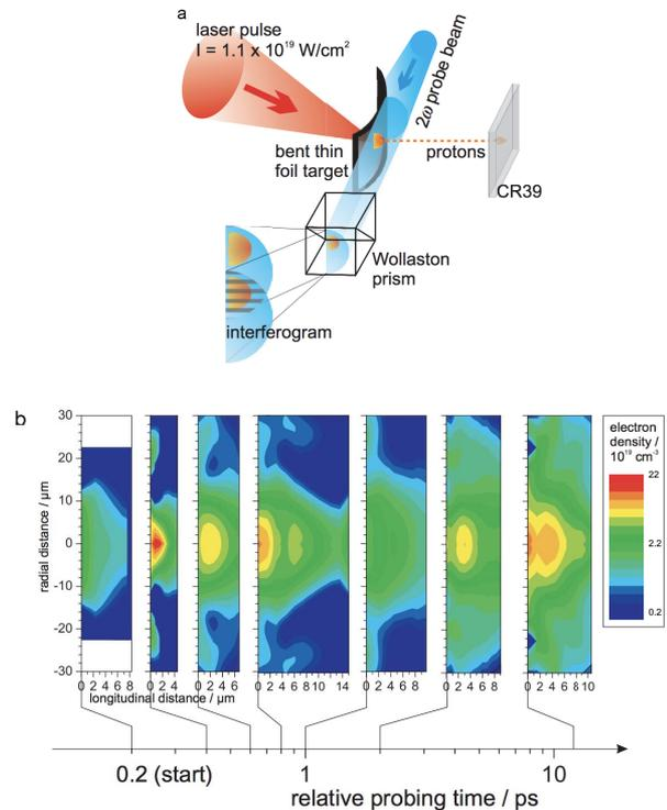
**Figure 1.** Electron density interferometric measurement. (a) Schematic overview of the experimental diagnostic setup. (b) Temporal evolution of the electron density at the rear surface of the target. All pictures are shifted +200 fs due to the logarithmic timescale. Figure from Ref. [24].
