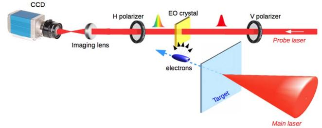
**Figure 11.** Sketch of the experimental setup. The FLAME laser is focused on a stainless steel target ejecting a relativistic electron beam able to escape from it as well as EMPs. These two interaction products induce local birefringence on a ZnTe electro-optic crystal, such that a linearly polarized laser, crossing the crystal, can probe them<sup>[28]</sup>.
