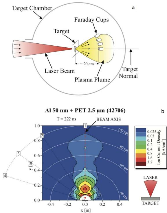
**Figure 6.** (a) Sketch of the experimental setup at the PHELIX sub-picosecond laser facility. (b) Spatial distribution of ion current density using a double-layer target with Al on the front side and PET on the rear side irradiated with 516 J of laser energy.
