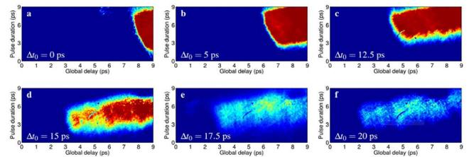
**Figure 16.** Evolution of the EM radiation pulse emitted by the target. By focusing the main laser onto a wedged target, the probe laser is sent onto the ZnTe crystal with different delays. The horizontal axis represents the relative probe arrival time ( $t$ ) associated with each pixel<sup>[31]</sup>.  $\Delta t_0$  is the delay between the main and probe laser pulses. From Ref. [31].
