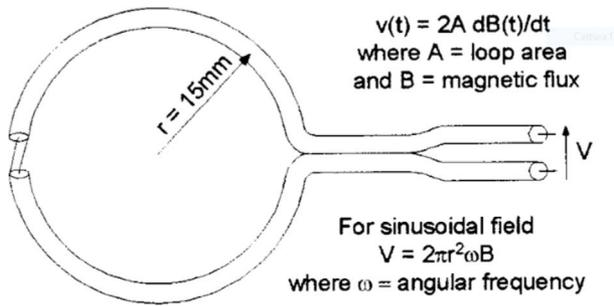
Figure 4. Moebius loop antenna layout. Figure from Ref. [14].
