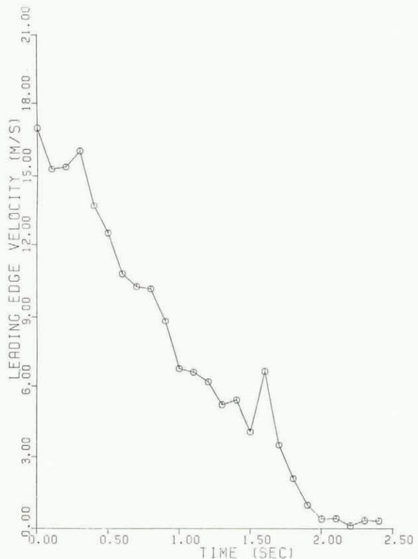
Fig.8. Velocity of the leading edge versus time (computer).
