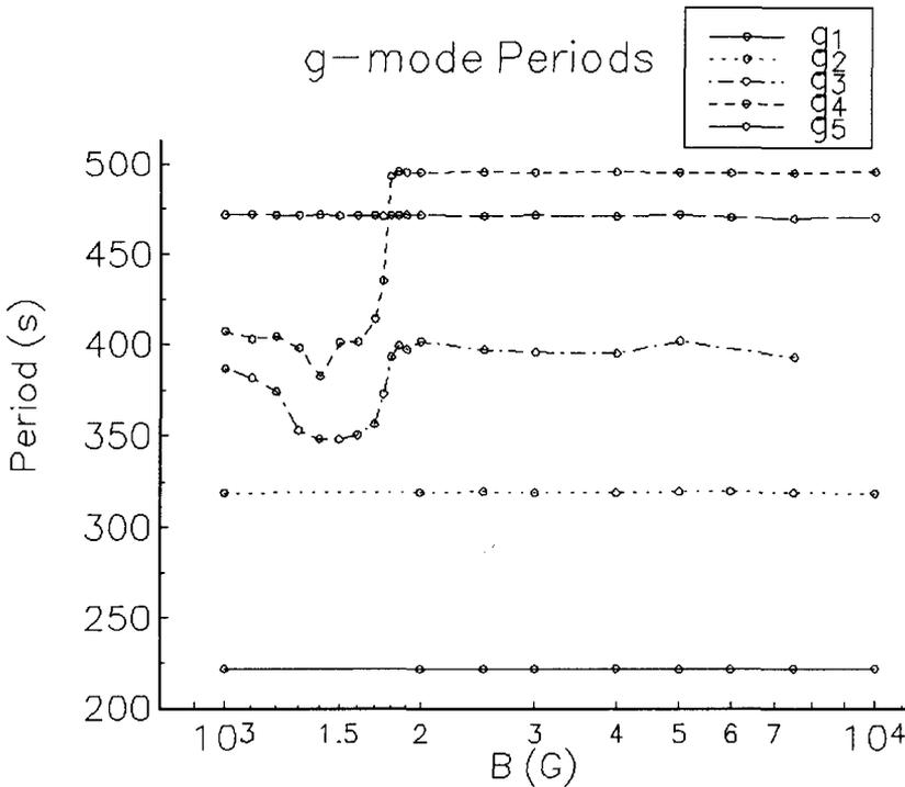
**Figure 1** Pulsation periods of  $g_1 - g_5$  modes with  $\ell = 2$  for a compositionally stratified  $0.6 M_\odot$  white dwarf model ( $T_e = 9960$  K,  $M_{\text{He}}/M_\star = 10^{-5}$ ,  $M_{\text{H}}/M_\star = 10^{-10}$ )
