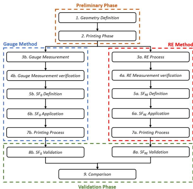
Figure 1. Methodology for validating dimensional shrinkage compensation in AM processes using RE method and Gauge method (benchmark method)
