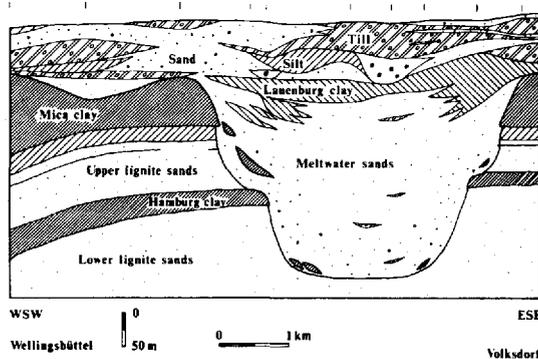
Fig. 6. Cross-section through a deeply incised tunnel valley in the Miocene mica clay and lignite sands in Hamburg-Volksdorf.
