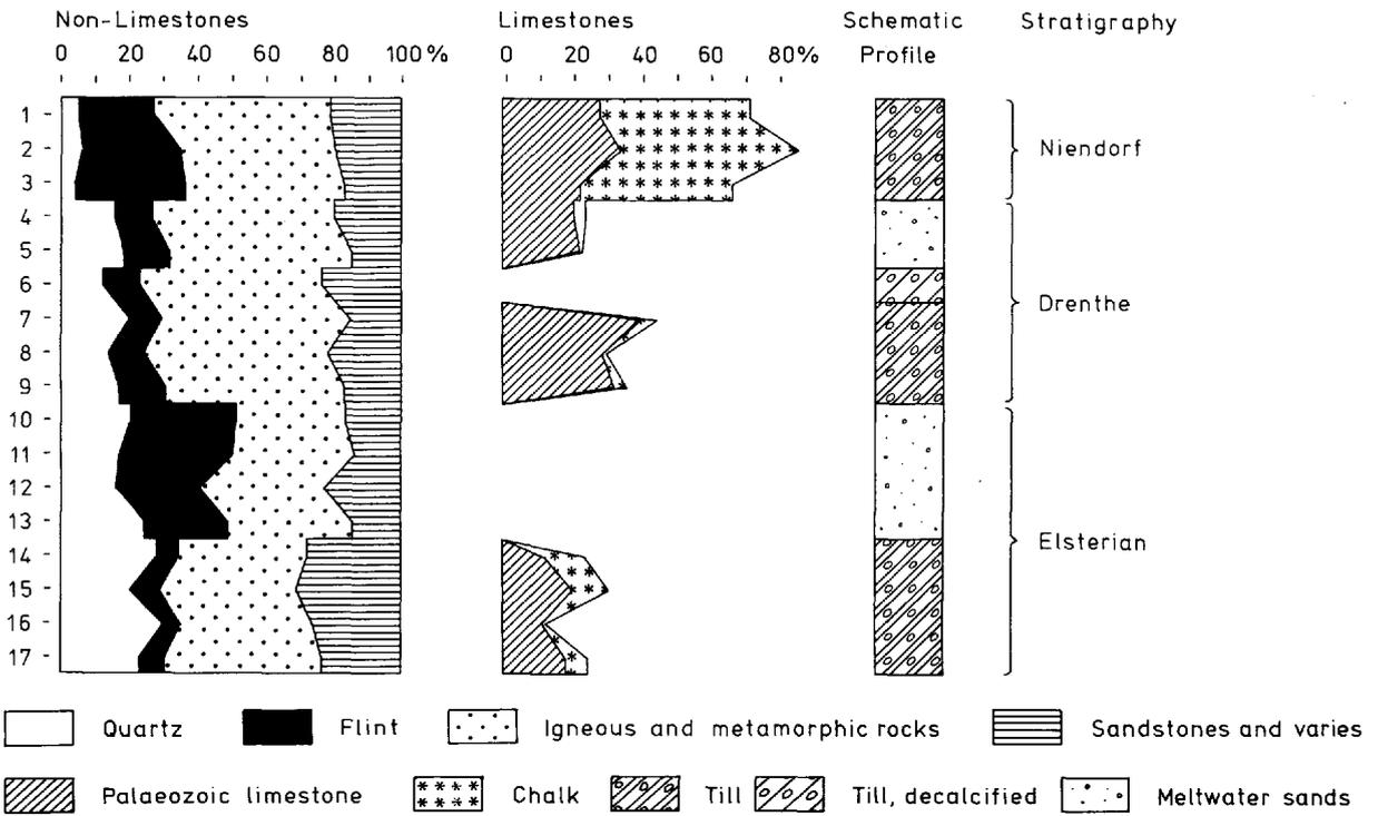
Fig. 2. Fine-gravel analysis of the Pleistocene sequence in the Hemmoor chalk quarry (fraction 3 to 5 mm). Almost no glacier erosion has taken place (Ehlers 1979).
