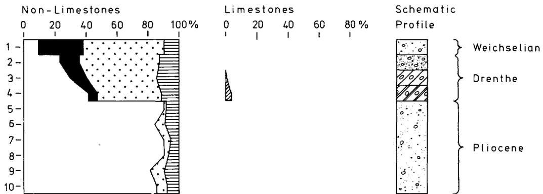
Fig. 3. Fine-gravel analysis of a drilling in Hamburg-Eidelstedt. The underlying Pliocene quartz sands have been considerably reworked and incorporated in the Drenthe till, which usually contains only about 10% quartz in this area.
