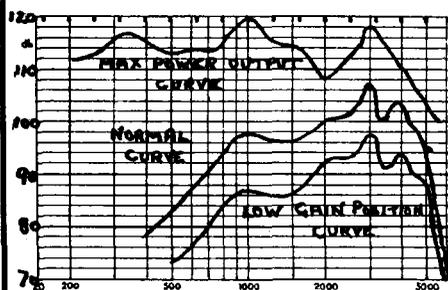
Frequency Response 500 - 5000 cps. Maximum Amplification (at 3000 cps) 46 dB. Maximum power output (1000 cps) 120 dB.
