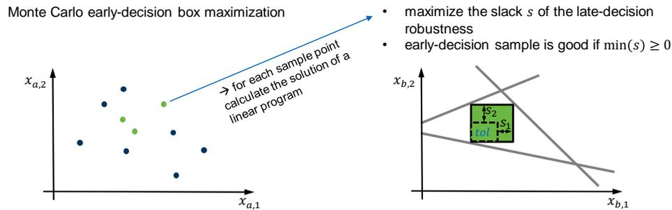
Figure 2. Schematic representation of the hybrid SCSBT algorithm; left: Monte Carlo early-decision solution box maximization; right: linear program for maximizing the slack  $s$  of the late-decision flexibility
