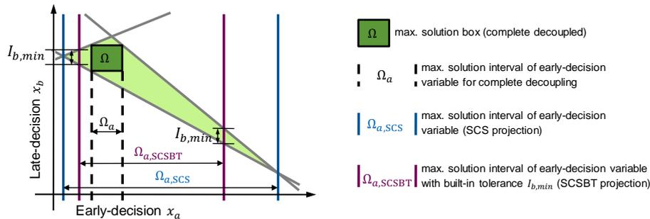
**Figure 1. Complete decoupled solution box, early-decision solution space projection by both, SCS and SCSBT**
