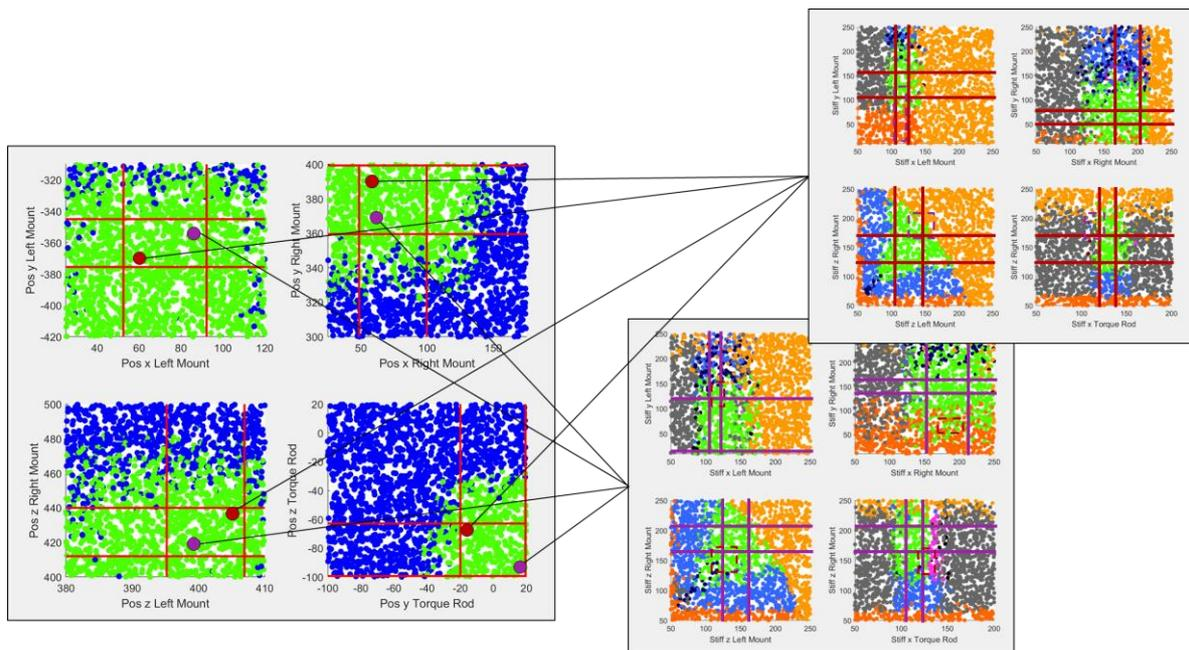
**Figure 5. Solution-compensation space projection with built-in tolerance: maximized solution box of mount positions (left) and emerging solution boxes for mount stiffnesses (right); shown are two possible mount positions (red and violet points left), which lead to different late-decision solution boxes (right); green dots represent good design points, other colors indicate violation of at least one requirement**
