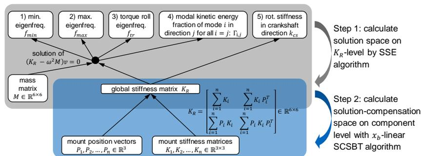
**Figure 4. Quantities of interest of a powertrain mount system (1-5) and the two-step top-down approach to calculate SCSBT on component level with the mount positions and stiffnesses as early- and late-decision variables, respectively**
