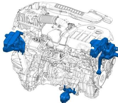
**Figure 3. Powertrain system including combustion engine, electric drive unit and gearbox as well as highlighted left mount, right mount and torque rod**
