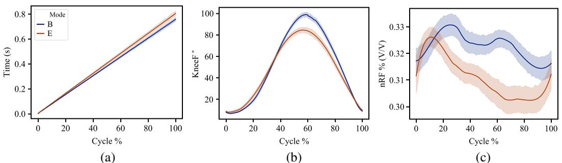
**Figure 4.** The averaged user behavior in *B* and *E* modes across all subjects and squat cycles. All data were segmented into squat cycles and normalized to the same cycle percentage. 4a represents the timing information of each mode. 4b shows the knee flexion angles in each mode. 4c shows the muscle activation magnitude of the rectus femoris in each mode, normalized in magnitude to the maximum value in *B*.
