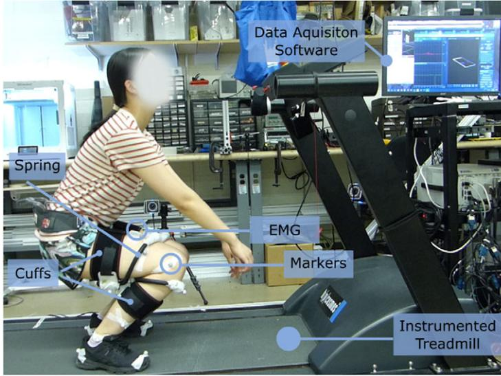
**Figure 3.** A user performing a squat in the SpringExo passive exoskeleton. The instrumented treadmill is used to collect foot pressure and loading data. The motion of the human body is captured using infrared markers. Surface EMG signals are used to collect muscle activation data.
