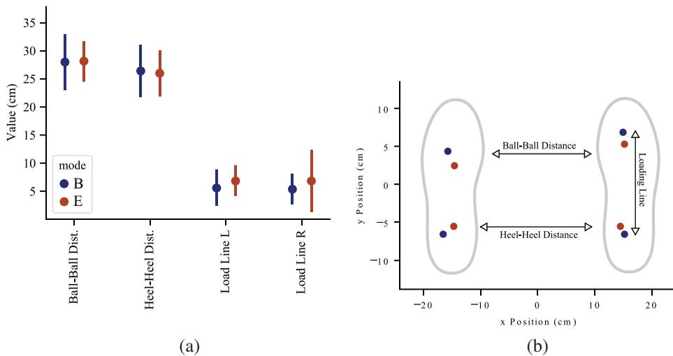
**Figure 6.** Foot loading behavior of the user with the exoskeleton donned and doffed. 6a shows the effect between each mode, B and E on the loading of the feet across all subjects. The variables shown are the distances between the balls and heels of the right and left feet, as well as the length of the pressure loading lines of each foot. 6b shows a visual representation of these variables.
