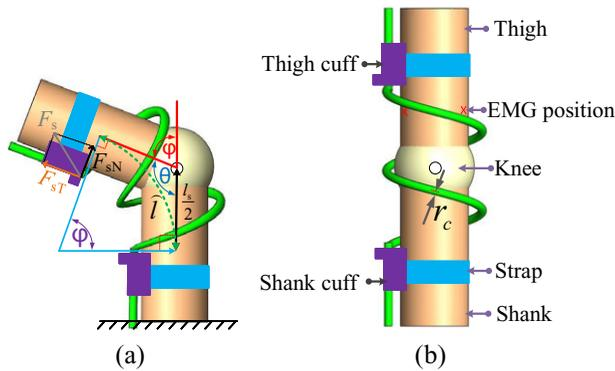
**Figure 2.** A kinematic diagram of the SpringExo donned on the leg. The leg is flexed at an angle  $\phi$  with SpringExo donned (a) and the resulting Force  $F_s$  that can be decomposed into the normal and tangential components  $F_{sT}$  and  $F_{sN}$ . The original state of the upright leg with the SpringExo donned (b) with the mechanical components that make up the SpringExo.
