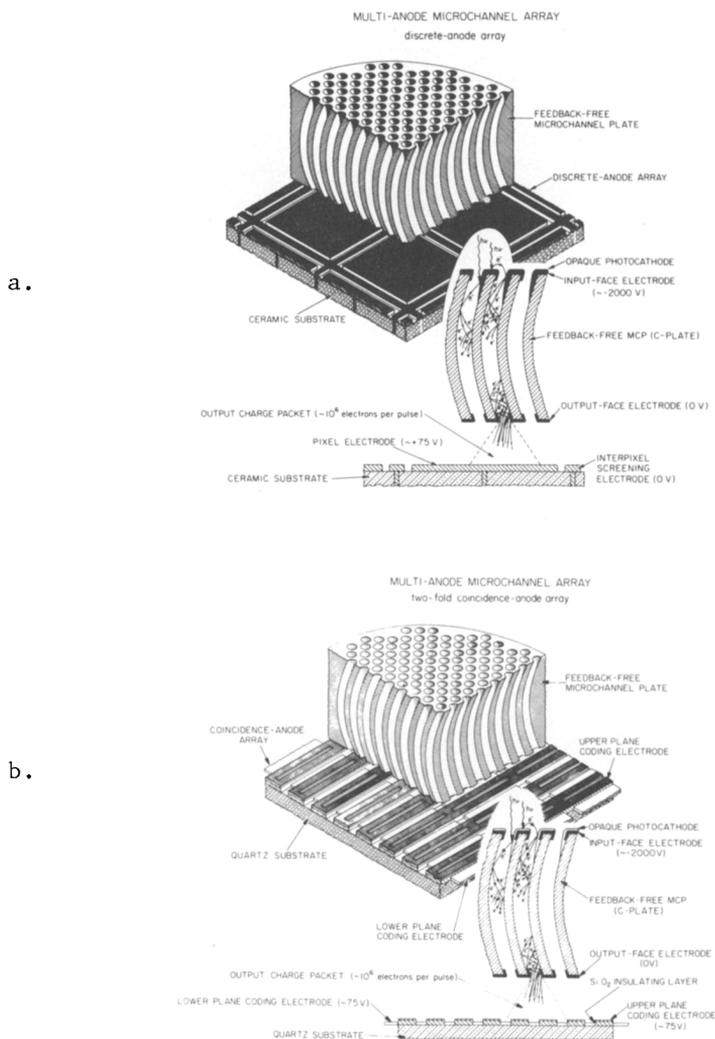
Figure 1. Schematics of Multi-Anode Microchannel Array Detectors.
