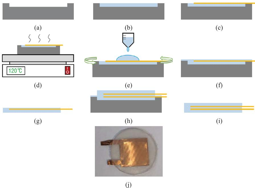
**Figure 3.** The fabrication process of capacitor. (a) printing 3D molds, (b) pouring Ecoflex, (c) placing copper electrodes, (d) curing, (e) spin-coating Ecoflex, (f) curing, (g) removing the mold, (h) bonding the two-halves structures, (i) curing and removing the mold, and (j) capacitor picture.
