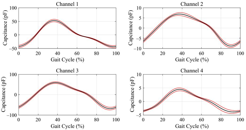
**Figure 5.** The normalized capacitive sensing signals. (a)–(d) represent 4 channels’ capacitive sensing signals. The black solid curves denote the mean of capacitive sensing signals of 50 gait cycles. The red solid lines denote the mean  $\pm$  standard deviation. The gait cycle starts at the heel strike and ends at the next heel strike, corresponding to the gait percent from 0 to 100% (shown in the horizontal axis). Data come from subject 1 walking at normal speed.
