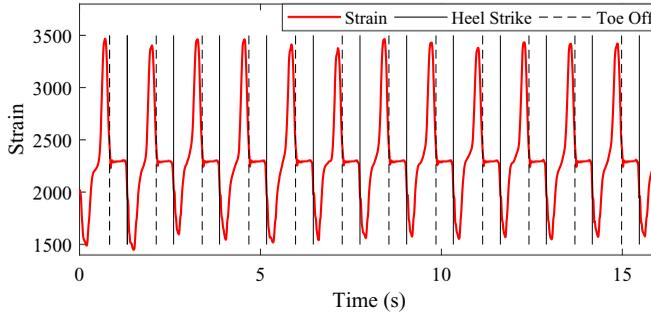
**Figure 6.** The strain signals of prosthetic foot at normal walking speed (subject 1). The red solid curve denotes the strain signal. The black dashed and solid lines denote the gait events: heel strike and toe off, respectively.
