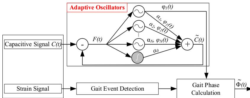
**Figure 4.** The framework of gait phase estimation (adapted from Gams et al., 2009; Yan et al., 2017; Xu et al., 2020b). The capacitive sensing signals are input to the AOs. The strain signals of prosthetic foot are used to detect gait events.
