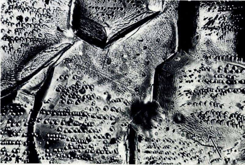
*Fig. 1. Rows of etch pits in a stressed crystal. Stress axis in direction of arrow ( $\times 200$ )*
