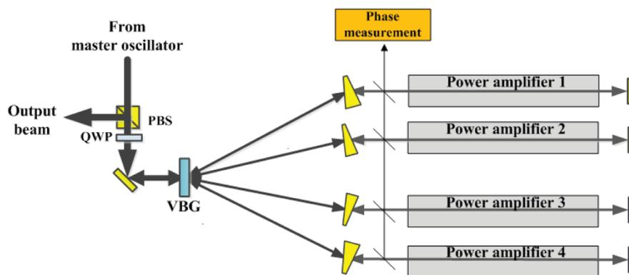
Figure 3. MOPA beam combination laser with the amplitude combining method using a VBG.
