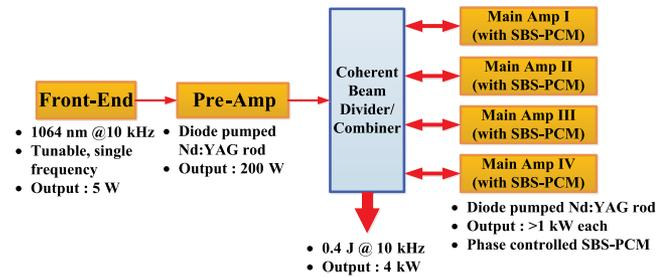
**Figure 1.** The schematic diagram of the Kumgang laser system.
