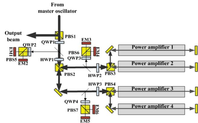
**Figure 2.** The MOPA beam combination laser with the amplitude combining method using PBS: EM1–EM6, energy meters.
