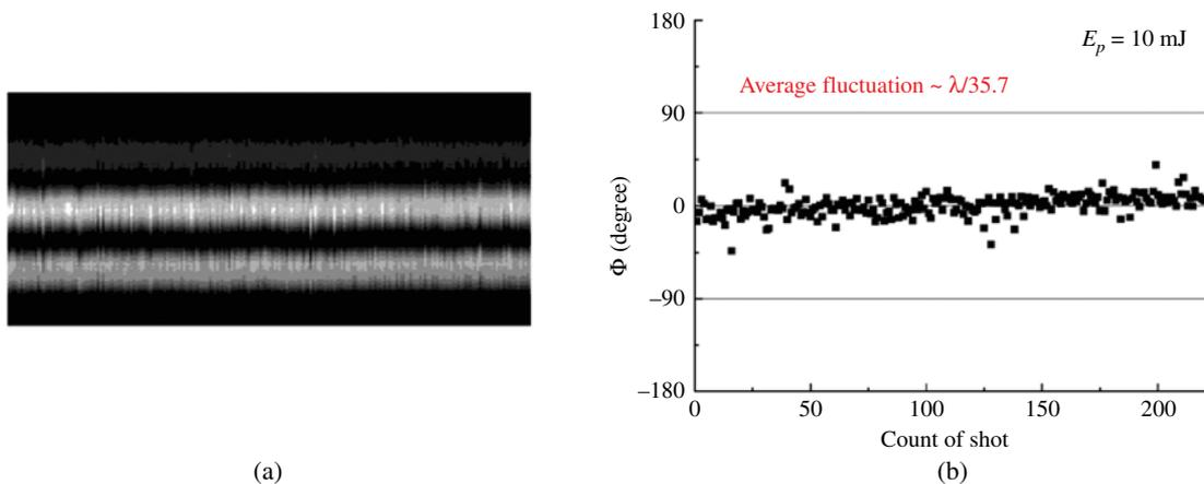
**Figure 6.** Experimental result of the self-phase-locked SBS-PCM. (a) A mosaic intensity pattern. It is generated by lining up one line of the intensity profile pattern recorded at each CCD image. (b) The measured relative phase. The standard deviation of the measured phase fluctuation is  $\lambda/35.7$ .
