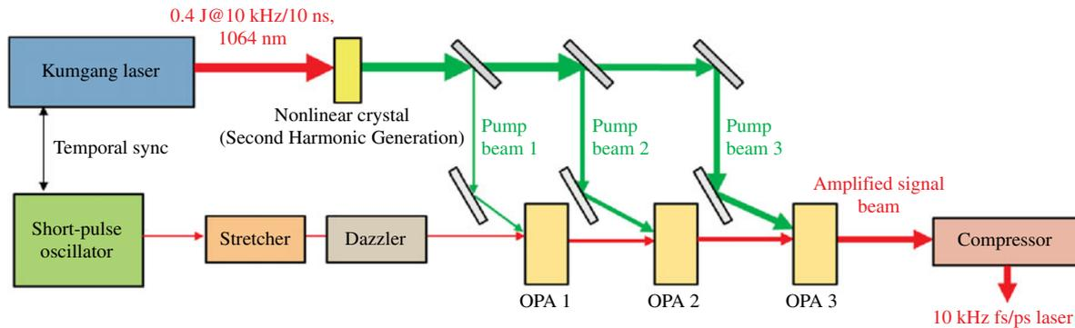
**Figure 17.** Schematic diagram of the generation of a fs/ps laser using the Kungang laser as a pump source: OPA1–OPA3, optical parametric amplifiers.
