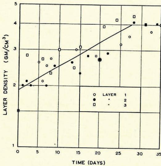
Fig. 6 (above). The dependence of the layer density on time
