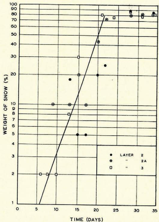
Fig. 7 (right). The increase with time in the amount of snow of grain size greater than 1 mm.
