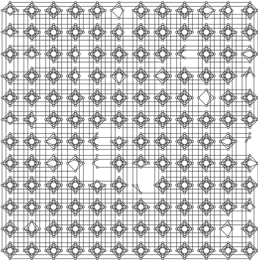
Fig. 1. Physical topology of LANL's D-Wave 2X.
