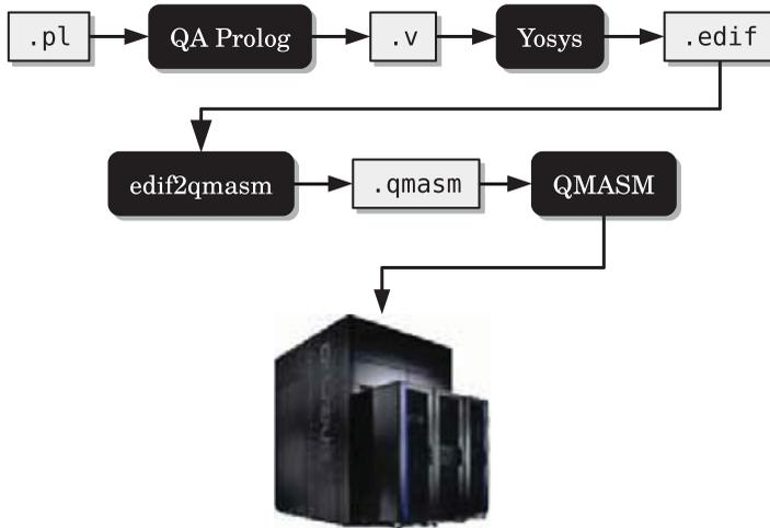
Fig. 5. Overall QA Prolog processing flow.
