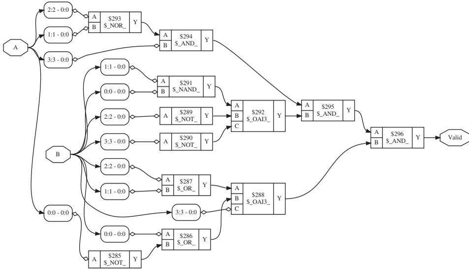
Fig. 12. Visualization of the optimized netlist Yosys produced from Figure 11.
