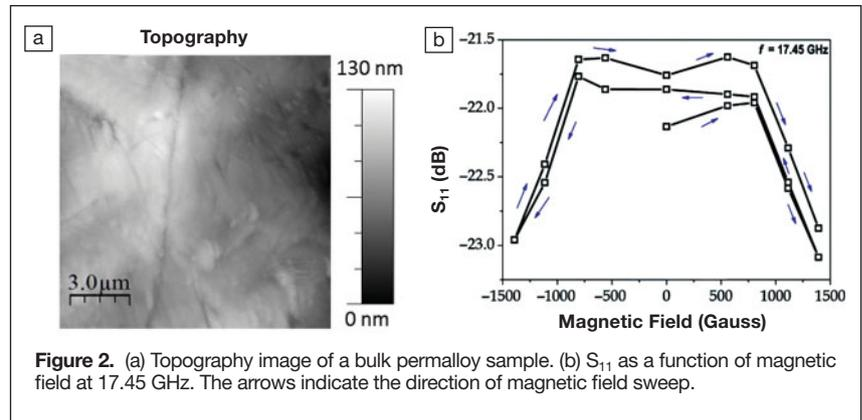
**Figure 2.** (a) Topography image of a bulk permalloy sample. (b)  $S_{11}$  as a function of magnetic field at 17.45 GHz. The arrows indicate the direction of magnetic field sweep.
