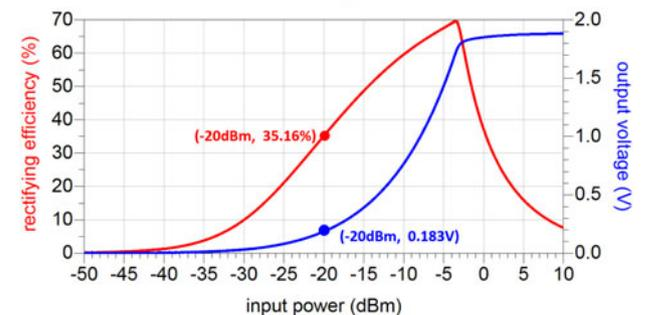
Figure 12. Topology and rectifying results for Skyworks 7630 diode (rectifying efficiency = 35.16%, output voltage = 0.183 V with  $-20$  dBm input power).
