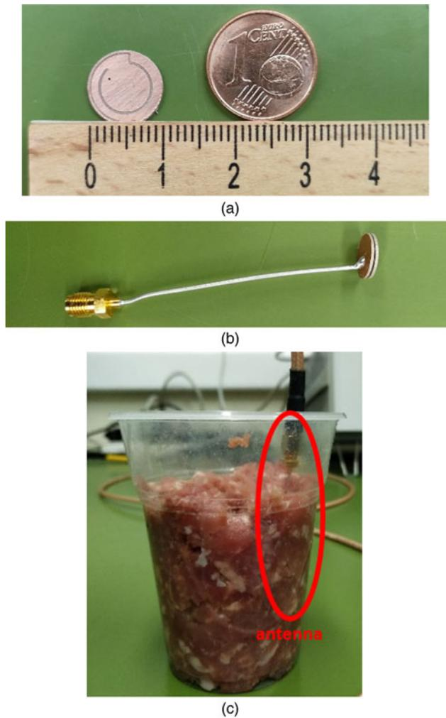
**Figure 13.** (a) Fabricated antenna comparing with one euro cent, (b) complete antenna with coaxial cable and superstrate and (c) antenna embedded into minced pork.
