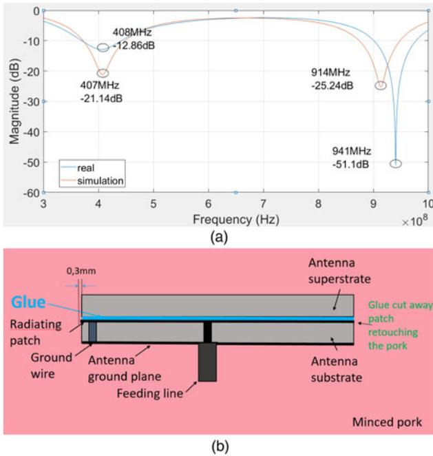
Figure 15. (a) Second measurement results and corresponding simulation when patch is expose to the minced pork meat and (b) corresponding experimental model.
