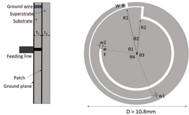
Fig. 1. The circular antenna.
