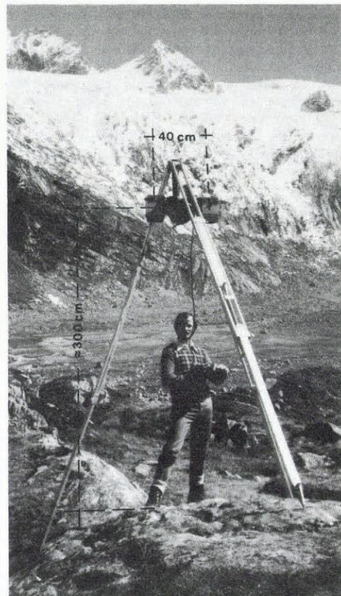
Fig. 7. The Wild C-40 wide-angle stereometric camera with a special tripod; in the pro-glacial area of Schwarzensteinkees.
