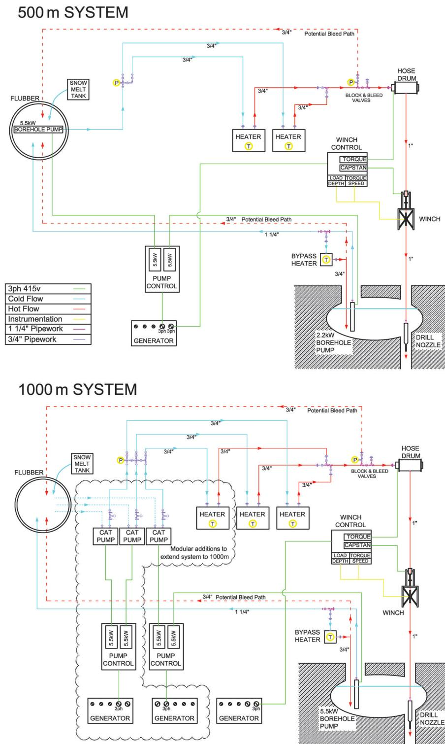
**Fig. 2.** The hot-water drill system for (a) up to 500 m ice depth and (b) up to 1000 m ice depth. The additional equipment required for the upgrade to 1000 m is inside the scalloped and dotted outline, and the 5.5 kW borehole pump is reused in the cavity.
