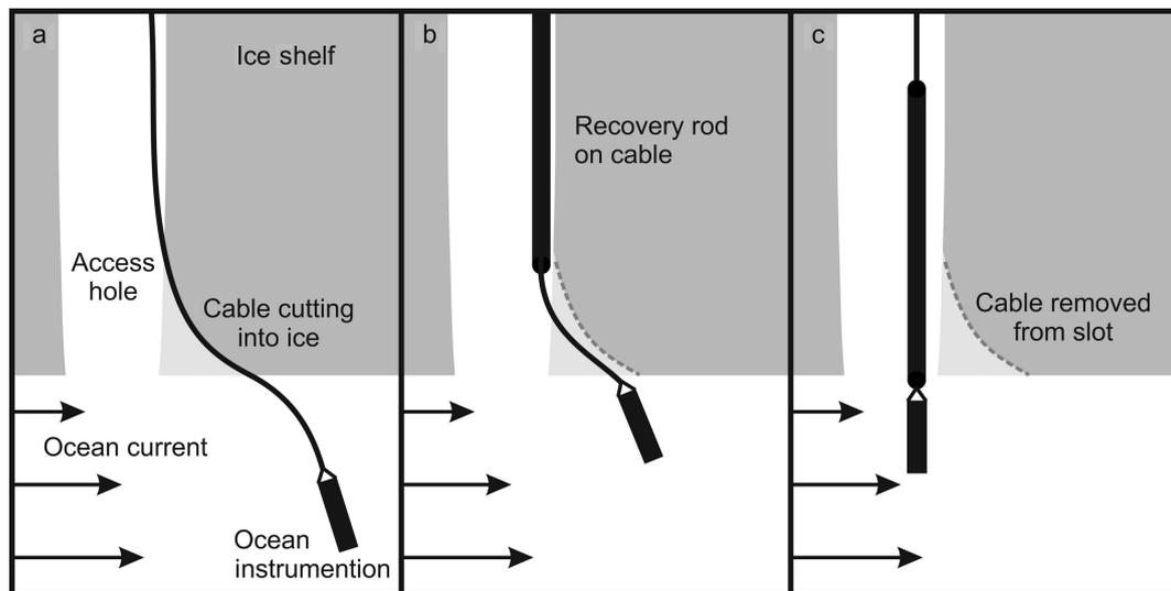
**Fig. 6.** Illustration of the recovery rod in operation. (a) The oceanographic instrument wire-cutting slot into the hole wall during profiling, (b) the recovery rod pushing the cable out of keyhole slot, and (c) the instrument ready for recovery into hole.
