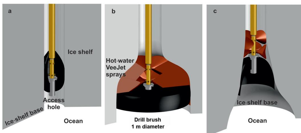
**Fig. 5.** Drill brush at the ice-shelf base (a) going down the hole with no hot water flow, (b) at the ice base and drilling upwards slowly and (c) at the ice base and drilling quickly before recovery up hole.
