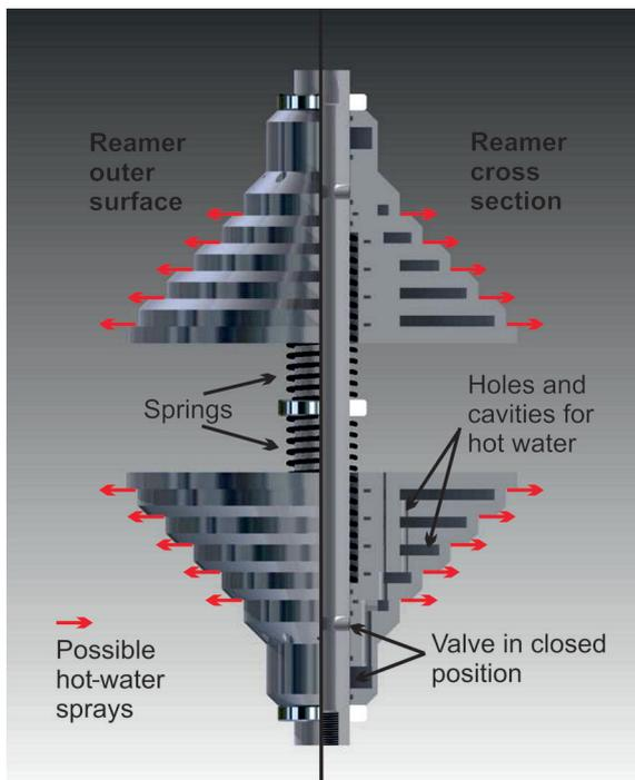
**Fig. 4.** Illustration of the reamer outer surface on the left and in cross section on the right. The red arrows indicate where water can spray from the reamer and the valve is shown in the off position.
