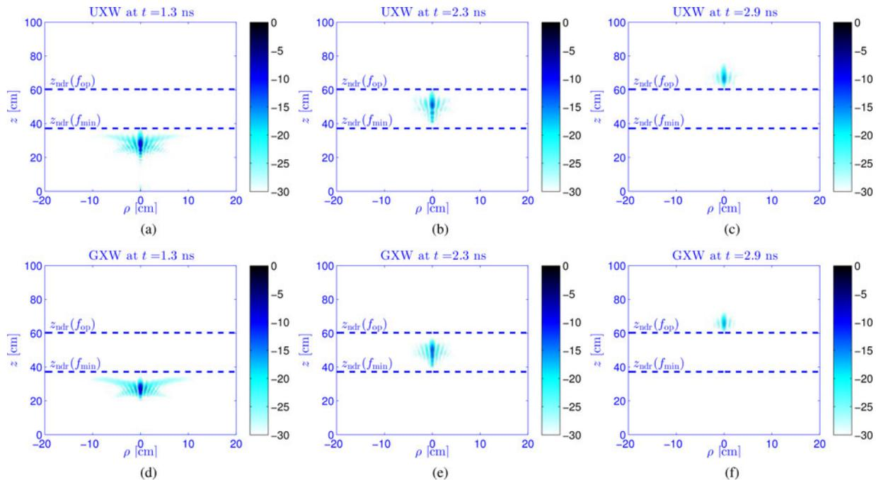
**Fig. 6.** Time evolution of (a)-(c) UXWs and (d)-(f) GXWs generated by means of focusing leaky waves. The intensity of  $\mathcal{E}_z(\rho, z; t)$  has been captured at (a) and (d)  $t=1.3$  ns, (b) and (e)  $t=2.3$  ns, (c) and (f)  $t=2.9$  ns, to show the distortion and the decay of the main spot of the pulse before and beyond the minimum and the operating nondiffractive ranges.
