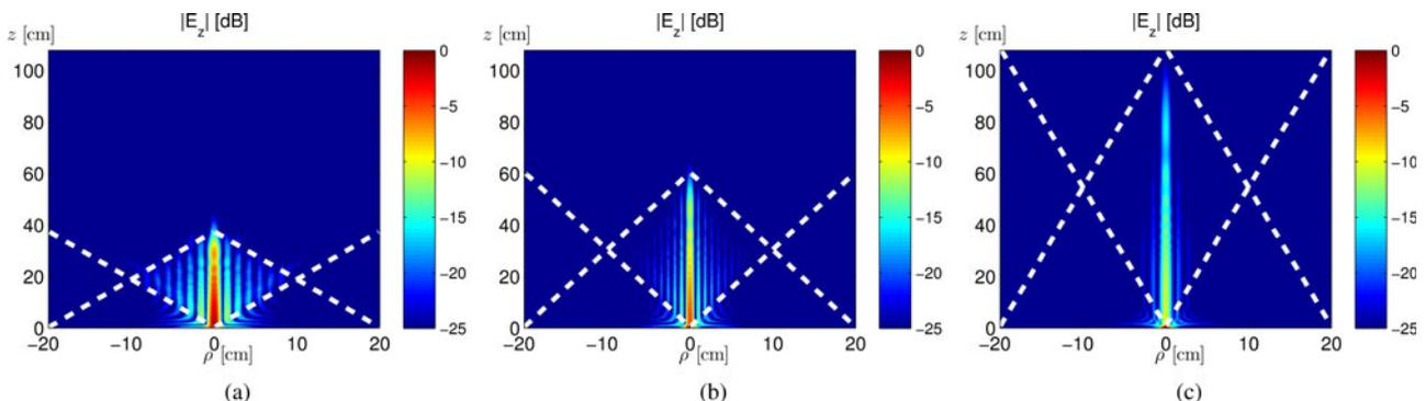
**Fig. 4.** Color maps of the normalized absolute value (in dB) of the  $E_z$  component of the electric field at (a)  $f=54$  GHz, (b)  $f=60$  GHz, and (c)  $f=66$  GHz, along an arbitrary  $\rho z$  plane limited by  $|\rho| < \rho_{ap}$  and  $0 < z < z_{ndr}(f_{max})$ . Due to the unavoidably dispersive character of the backward leaky wave, the shadow boundaries (white dashed lines) change as  $f$  and hence  $\beta_{\rho,-1}$  changes.
