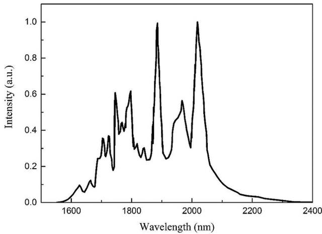
Figure 2. Fluorescence spectrum of a Tm:YAG crystal.
