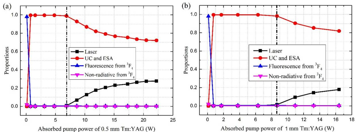
**Figure 9.** Proportions of all the transitions for (a) 0.5 mm Tm:YAG disk laser and (b) 1 mm Tm:YAG thick disk laser under the lasing condition.
