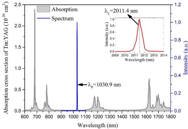
**Figure 4.** Absorption cross section of Tm:YAG and spectrum of pump light. Inset is the spectrum of output laser.
