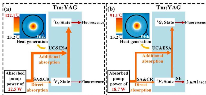
**Figure 7.** Operating principle diagram of the 0.5 mm Tm:YAG disk laser under (a) non-lasing and (b) lasing conditions. The thicknesses of the arrows are proportional to the intensities of the transitions.
