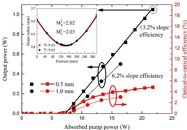
**Figure 6.** Output power of a Tm:YAG disk laser versus absorbed pump power for 0.5 and 1 mm thickness of gain medium. The inset shows the measured beam caustic and calculated beam quality at the output power of 1.05 W.
