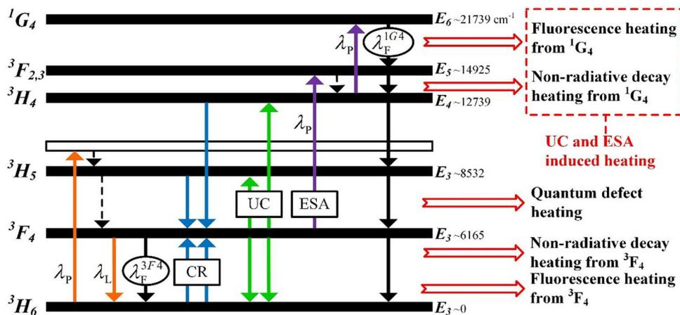
Figure 1. Energy diagram of a Tm:YAG crystal.
