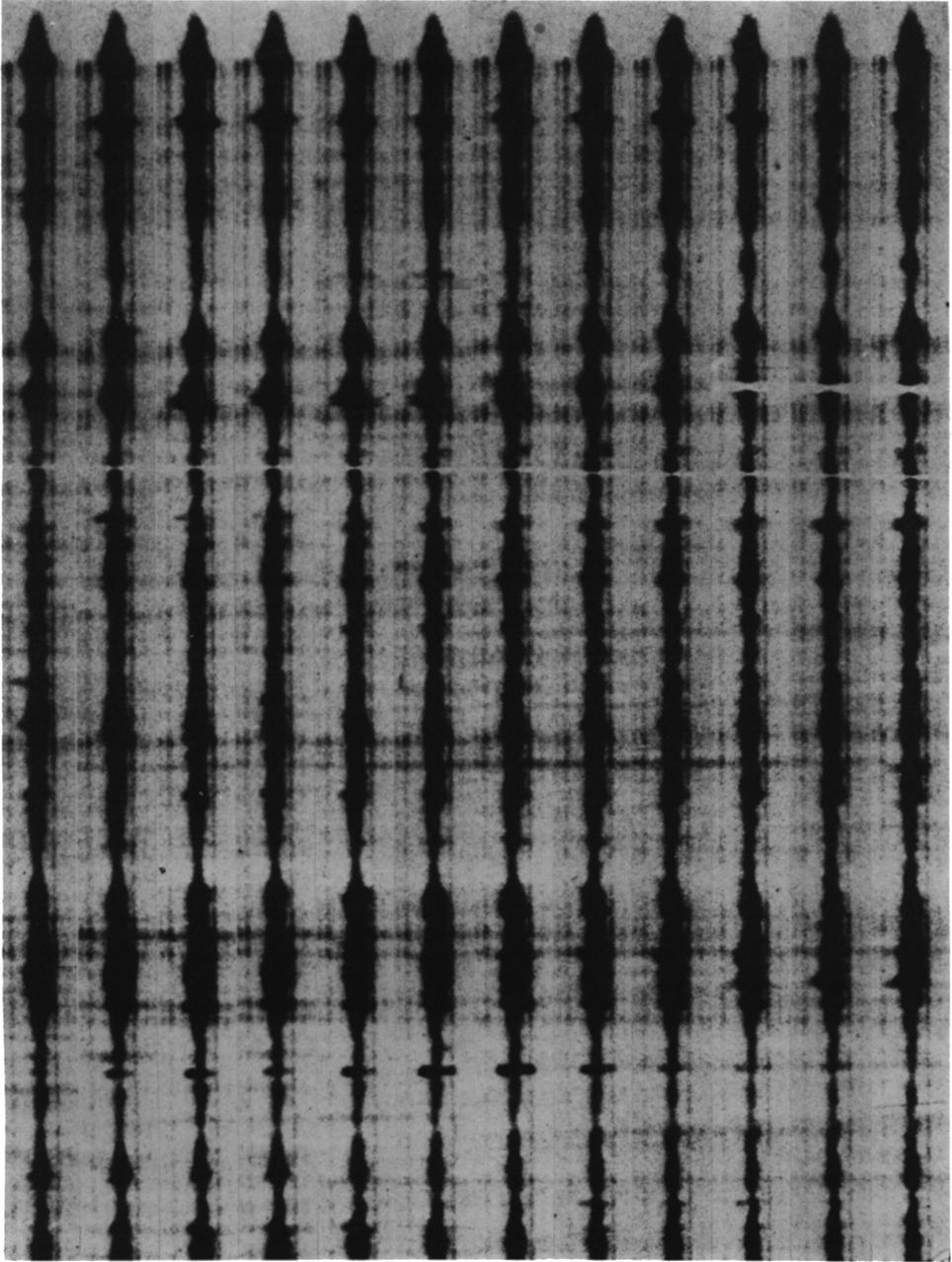
Fig. 4: Time sequence of C IV spectra taken in 20 second intervals. Solar limb is at the top, the spectra cover 1/2 of a solar radius.
