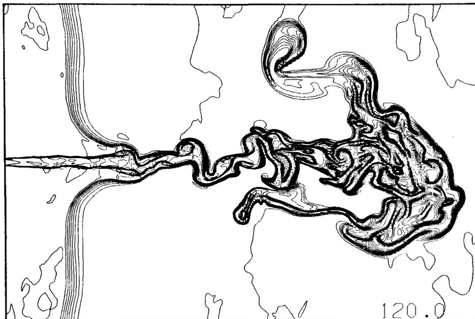
**Fig. 6** Disruption of a slab-symmetric supersonic ( $M=5$ ) jet caused by a rapid increase in ambient temperature. A 1% transverse perturbation is applied at the inlet (at left) with a sinusoidal time dependence at the resonant frequency of the slab [46]. The perturbation grows rapidly into large-scale kinks in the hot tenuous medium to the right of the temperature transition. A computational mesh of 750 longitudinal by 300 transverse zones is used; 20 zones span the initial slab width.
