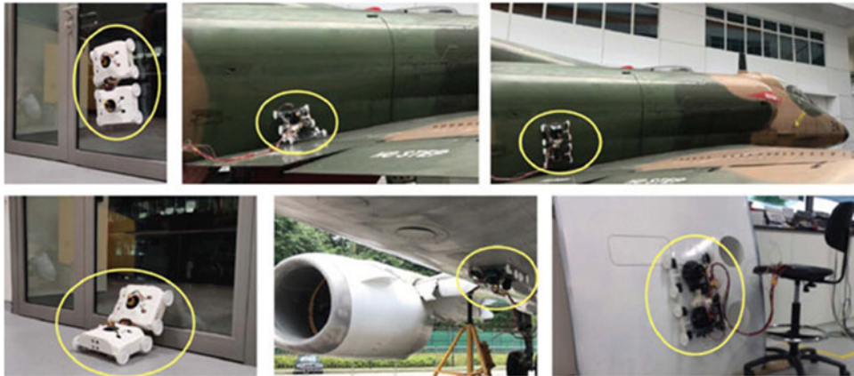
Figure 6. Reconfigurable climbing robot for visual inspection. Credit Balakrishnan Ramalingam et al. [36] (CC-BY).
