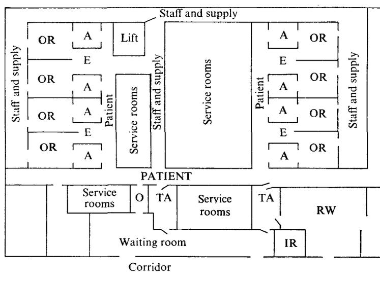
Fig. 1. Layout of the operating suite. A, Anaesthetic room; E, exit area; OR, operating room; TA, transfer area; IR, isolation room; RW, recovery ward; O, office.
