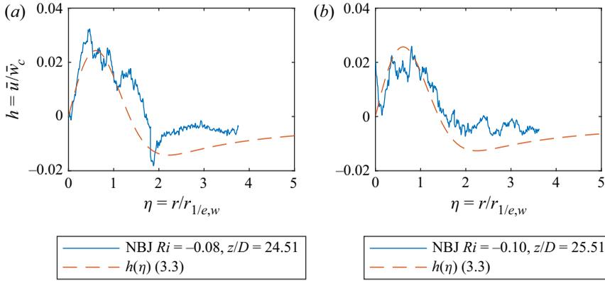
Figure 3. The shape function  $h$ , defined in (3.3), for the case of an NBJ with  $\lambda = 1.46$  and  $\delta_m \sim Ri$  (as defined by (4.1)) at  $Ri = -0.08$  in (a) and  $Ri = -0.10$  in (b). The corresponding normalised radial velocity profiles obtained in an experimental study by the present authors are also shown (Milton-McGurk *et al.* 2020, 2021).
