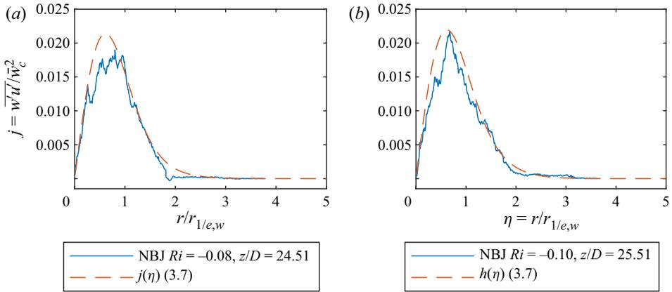
Figure 4. The shape function  $j$ , defined in (3.7), for the case of an NBJ with  $\lambda = 1.46$  and  $\delta_m \sim Ri$  (as defined by (4.1)) at  $Ri = -0.08$  in (a) and  $Ri = -0.10$  in (b). The corresponding normalised Reynolds stress profiles obtained in an experimental study by the present authors are also shown (Milton-McGurk *et al.* 2020, 2021).
