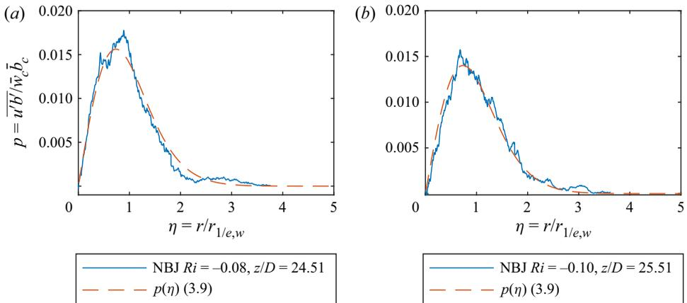
Figure 5. The shape function  $p$ , defined in (3.9), for the case of an NBJ with  $\lambda = 1.46$  and  $\delta_m \sim Ri$  (as defined by (4.1)) at  $Ri = -0.08$  in (a) and  $Ri = -0.10$  in (b). The corresponding normalised radial scalar flux profiles obtained in an experimental study by the present authors are also shown (Milton-McGurk *et al.* 2020, 2021).
