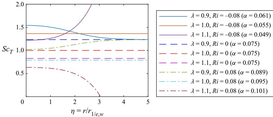
Figure 8. The turbulent Schmidt number,  $Sc_T$ , computed using (5.5), for several values of  $Ri$  and  $\lambda$  and a fixed  $\delta_m = -0.2$ . The corresponding value of  $\alpha$  implied by (2.14) is also shown.
