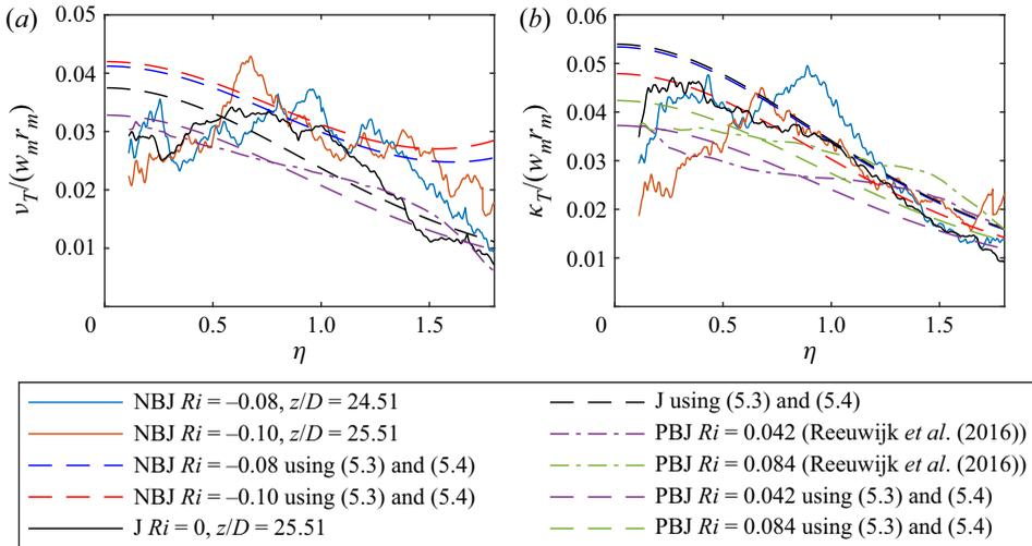
Figure 6. Non-dimensional turbulent momentum,  $v_T$ , and mass,  $\kappa_T$ , diffusivity calculated from the NBJ and J data obtained in Milton-McGurk *et al.* (2020, 2021) and PBJ data in van Reeuwijk *et al.* (2016). The analytical expressions given in (5.3)–(5.4) are also shown.
