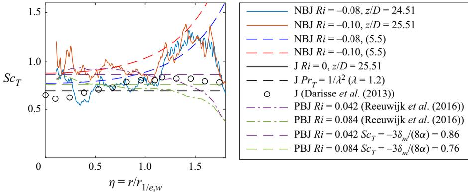
Figure 7. The turbulent Schmidt number,  $Sc_T$ , calculated from the NBJ and J data obtained in Milton-McGurk *et al.* (2020, 2021) and PBJ data in van Reeuwijk *et al.* (2016). The analytical expressions, as implied by (5.5), are also shown.
