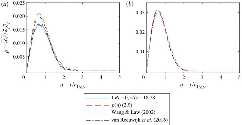
Figure 1. The shape function  $p$ , defined in (3.9), for the case of a neutral jet ( $\lambda = 1.2, \delta_m = -0.20$ ) in (a), and pure plume ( $\lambda = 1.0, \delta_m = -0.20$ ) in (b). The corresponding normalised radial scalar flux profiles obtained in an experimental study by the present authors (jet only) (Milton-McGurk *et al.* 2020, 2021), as well as by Wang & Law (2002) and van Reeuwijk *et al.* (2016), are also shown.
