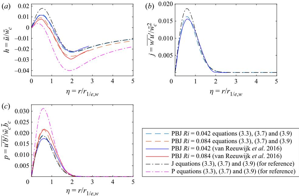
Figure 2. The shape functions  $h, j$  and  $p$  defined in (3.3), (3.7) and (3.9), respectively, are shown in (a)–(c) for the case of a PBJ with  $\lambda = 1.0$  and  $\delta_m = -0.175$  at  $Ri = 0.042$  and  $Ri = 0.084$ . The corresponding normalised radial velocity, Reynolds stress and radial scalar flux profiles obtained from DNS study by van Reeuwijk *et al.* (2016) are also shown in each case. The analytical expressions for a pure jet (J) and plume (P) are also shown as a reference.
