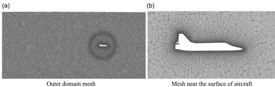
**Figure 3.** Unstructured grid for inner and outer domains.
