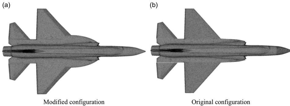
**Figure 2.** Surface mesh of modified and original configuration.
