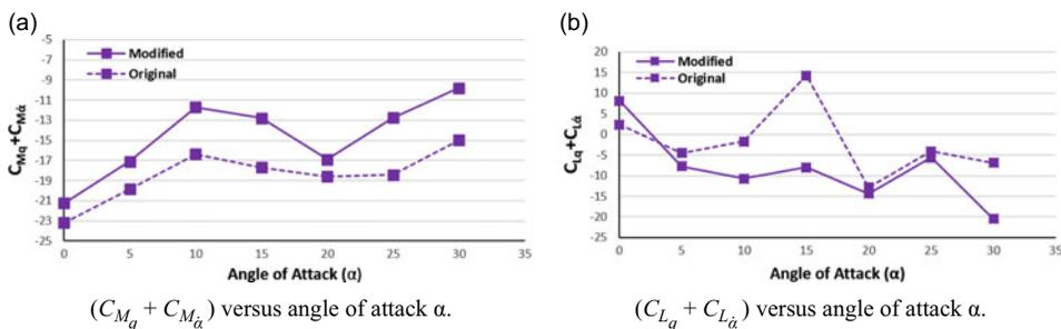
**Figure 15.** Damping coefficients at  $Ma = 0.6$ .
