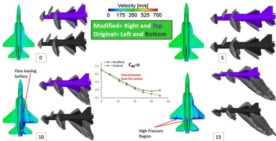
**Figure 14.** Flow visualisation at Mach = 1.4. The left part of the velocity flow on the aircraft and the bottom shock wave representation is original, and the right part of the velocity flow on the aircraft and top shock wave representation is modified.
