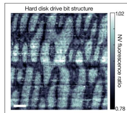
Nitrogen-vacancy (NV) magnetometry image of the bits of a hard disk at  $T = 6$  K. Dark features correspond to the 5.3 G magnetic field contours (2892 MHz RF field). Scale bar, 100 nm. Credit: *Nature Nanotechnology*.
