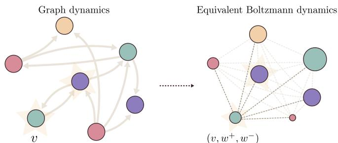
**Figure 2.** Visual representation of the equivalence between the network dynamics and the equivalent Boltzmann one. A situation in which the interactions between the agents are regulated by a network structure (left panel) is replaced, without approximation, by one in which every agent can interact with any other agent (right panel).
