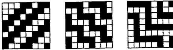
Figure 3. The design of a twill of exact order eight and its colouring by thin striping to produce the prefabric patterns 4-1-1\* and 8-5-1\*.
