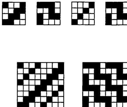
Figure 4. The designs of two twills of exact order four and one of exact order eight, all of which can be thinly striped to produce the pattern 4-1-1\*.
