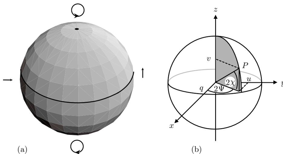
Figure 2—The Poincaré sphere, with the circular polarisations indicated at the poles and the linear polarisations at the equator; (b) the parameters  $\Psi, \chi, q, u, v$  for an arbitrary point  $P$  on the sphere.
