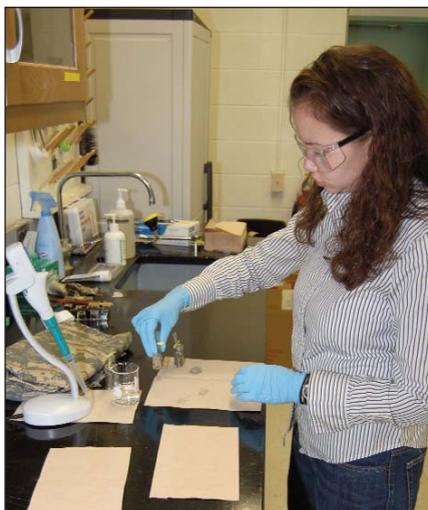
Christina Diaz, a doctoral candidate at Cornell in Juan Hinestroza's group, prepares nylon-cotton camouflage fabric coated with colloidal polystyrene particles through convective and electrostatic self-assembly. Her goal is to make the fabric invisible to someone wearing night vision goggles.
