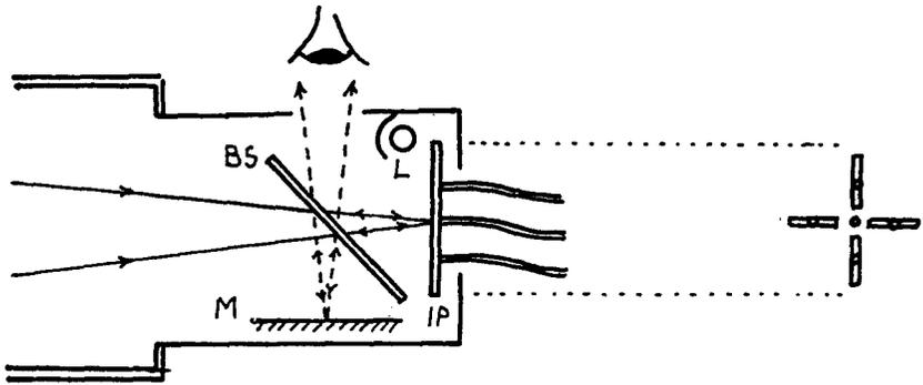
Figure 1. Schematic diagram of the adaptor. BS: beam splitter, M: mirror, IP: input plate with fibre ends, L: small lamp
