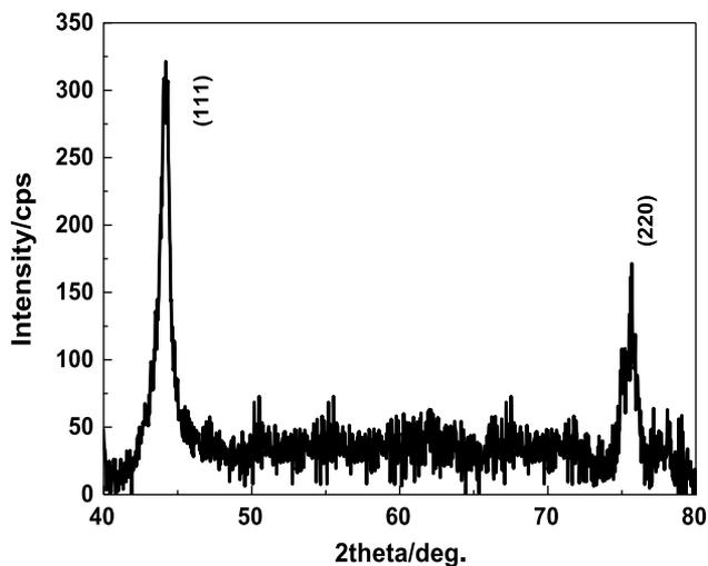
Figure 9. XRD pattern of HDC shell.
