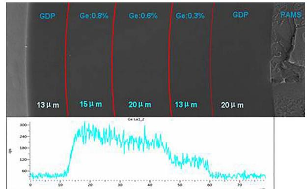
**Figure 3.** Cross-sectional SEM image and EDS results of GDP shell graded doped with Ge.
