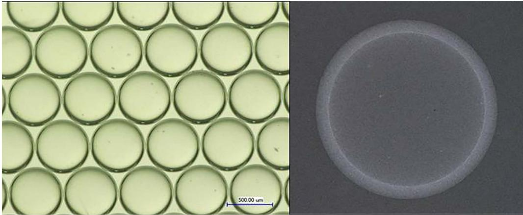
**Figure 7.** Microphotograph of batch PS shells and computed tomography image of individual PS shell.
