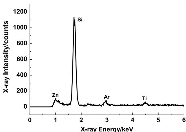
Figure 6. XRF spectrum of an argon filled Si:GDP.
