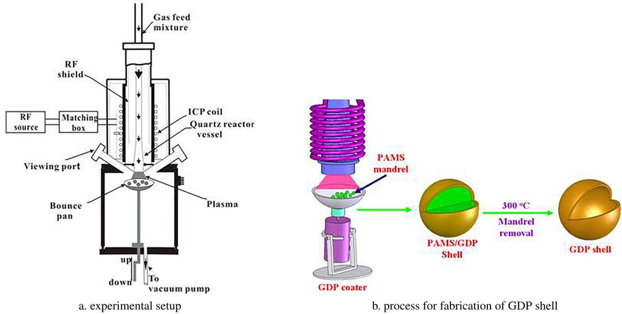
**Figure 1.** Experimental setup and schematic process for fabrication of GDP shell.
