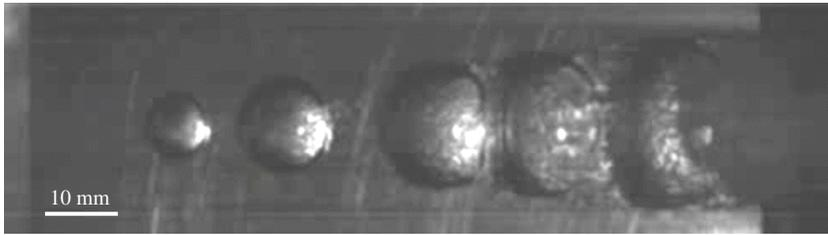
FIGURE 2. Streak cavitation on NACA0009 hydrofoil. The flow is from left to right with a frequency of bubble generation of 1000 Hz. The image was taken with an exposure time of 55  $\mu$ s. The cavitation number is  $\sigma = 5.4$  and the Reynolds number is  $Re = 1.1 \times 10^5$ . The image was taken at the cavitation tunnel of the Laboratory for Hydraulic Machines/École polytechnique fédérale de Lausanne by the authors.
