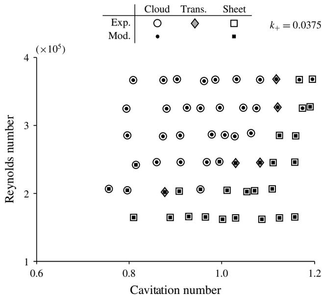
FIGURE 7. Stability map for sheet and cloud cavitation for  $k_+ = 0.0375$ . The map shows operation points where sheet (squares) and cloud cavitation (circles) occur. Operation points marked with diamonds could not be categorised. The larger symbols mark the experimental data, the smaller symbols are the results of the physical model (experimental data by Pelz *et al.* 2014).
