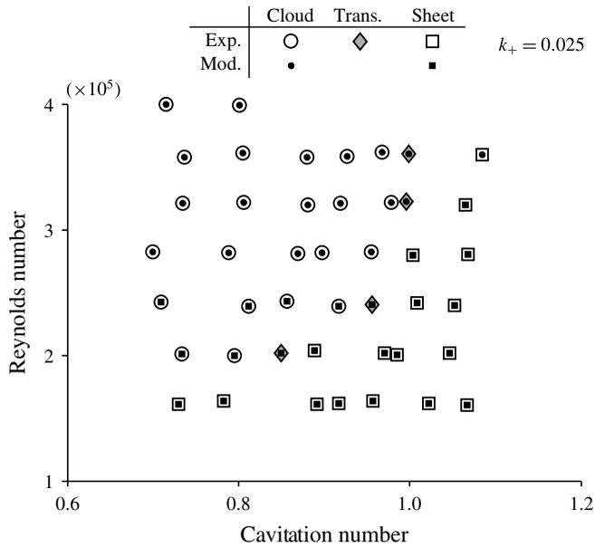
FIGURE 6. Stability map for sheet and cloud cavitation for  $k_+ = 0.025$ . The map shows operation points where sheet (squares) and cloud cavitation (circles) occur. Operation points marked with diamonds could not be categorised. The larger symbols mark the experimental data, the smaller symbols are the results of the physical model (experimental data by Pelz *et al.* 2014).
