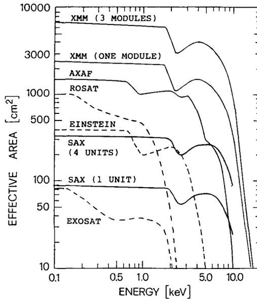
Fig. 2. Effective area of several X-Ray satellites.
