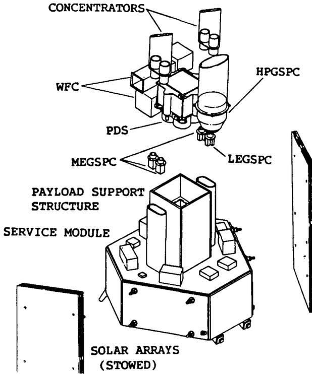
Fig. 1. SAX spacecraft and payload.
