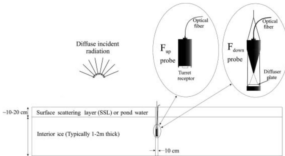
**Fig. 1.** Experimental configuration for profile observations. The up- or downwelling irradiance receptor probe was connected to the spectrophotometer by a 10 m long optical fiber. For each profile, the probe was lowered in 0.05–0.10 m increments down the hole to record irradiance vs depth.
