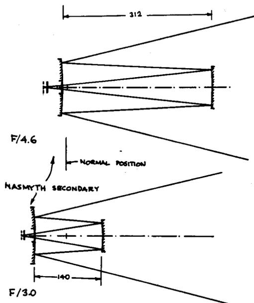
Figure 7. Meinel reflective prime focus field correctors utilizing the Nasmyth secondary mirror.
