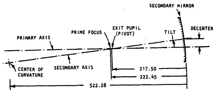
Figure 18. Definition of tilt and decenter errors for a secondary mirror. The primary mirror is to the right of the figure.
