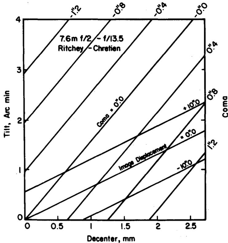
Figure 20. The zero coma condition with added loci for image displacement as function of secondary tilt and decenter.
