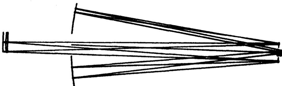
Figure 15. MacFarlane INCA II f/13.5 - f/3 focal reducer.
