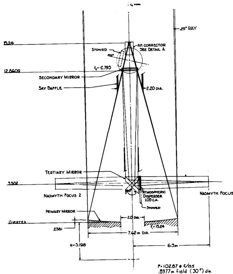
Figure 4. Optical configuration, baseline telescope design.
