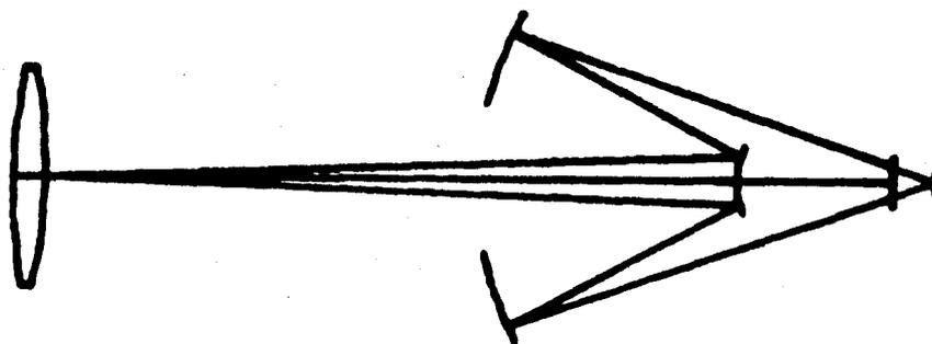
Figure 12. MacFarlane inverse Cassegrain focal reducer,  $f/1.5$ .
