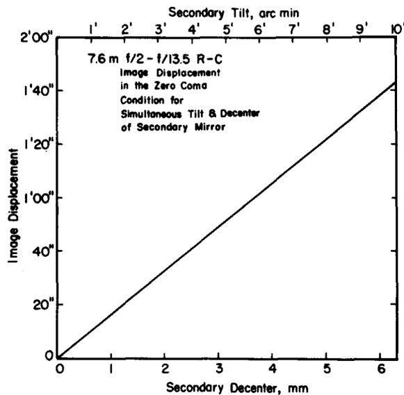
Figure 22. Illustrating a technique for correcting telescope pointing without introducing coma.
