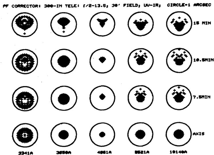
Figure 6. Spot diagrams for Fig. 5.
