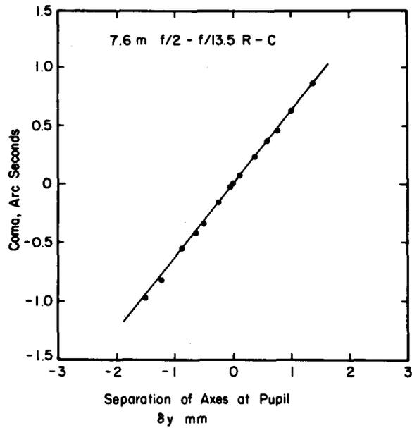
Figure 21. Numerical check of zero coma condition.
