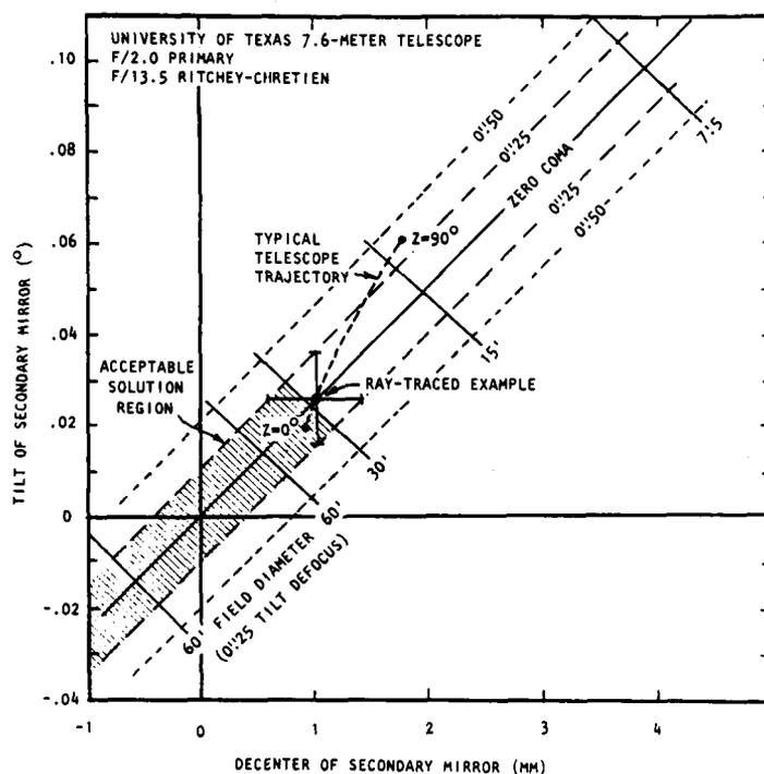
Figure 19. The zero coma condition for an f/13.5-f/2 R-C system.
