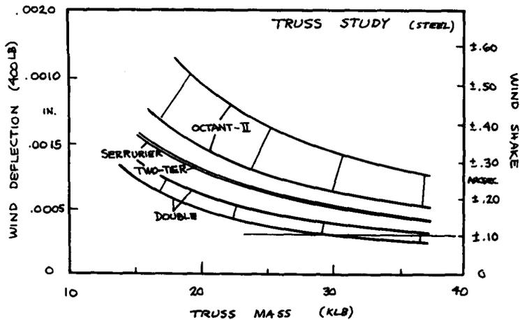
Figure 24. Deflection under gravity as function of weight of several truss geometries.
