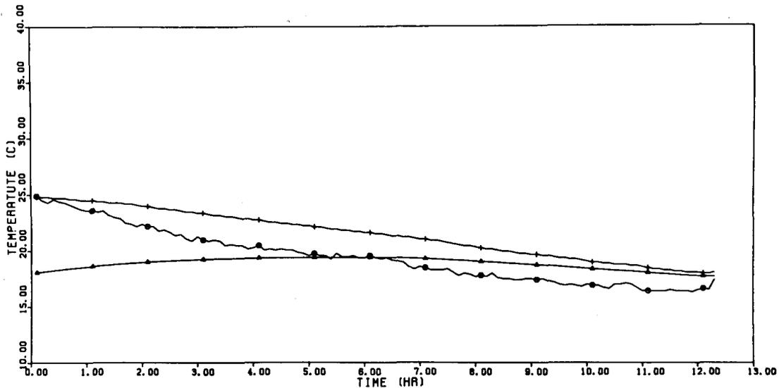
Figure 17. Variation of observatory air temperature (middle curve) during a 12 - hour nighttime period, together with computed mirror surface temperatures for a solid 12 cm thick blank. For the upper curve the initial temperature difference was zero; a 7 degree C temperature difference was assumed for the lower curve. Over the 12-hr period the average temperature difference, mirror minus air, was about the same (2 degrees) for both cases.
