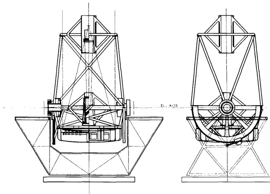
Figure 25. Structure concept for the 7.6-m telescope.
