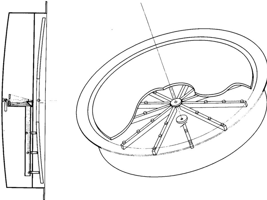
Figure 26. Illustrative layout of the laser figure control monitor system (Tull and Young, 1983).
