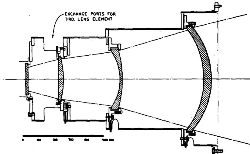
Figure 5. Richardson  $f/2$  prime focus field corrector.
