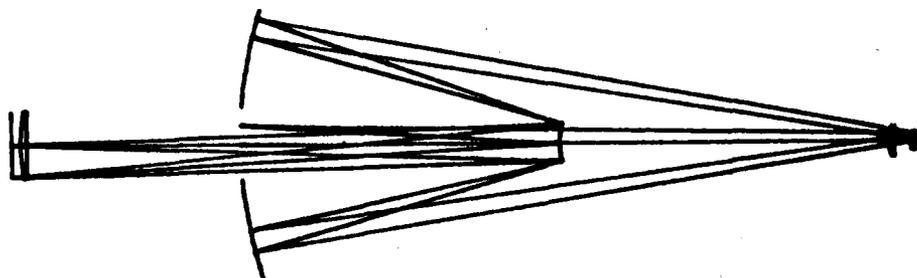
Figure 13. MacFarlane INCA f/13.5 - f/3 focal reducer.
