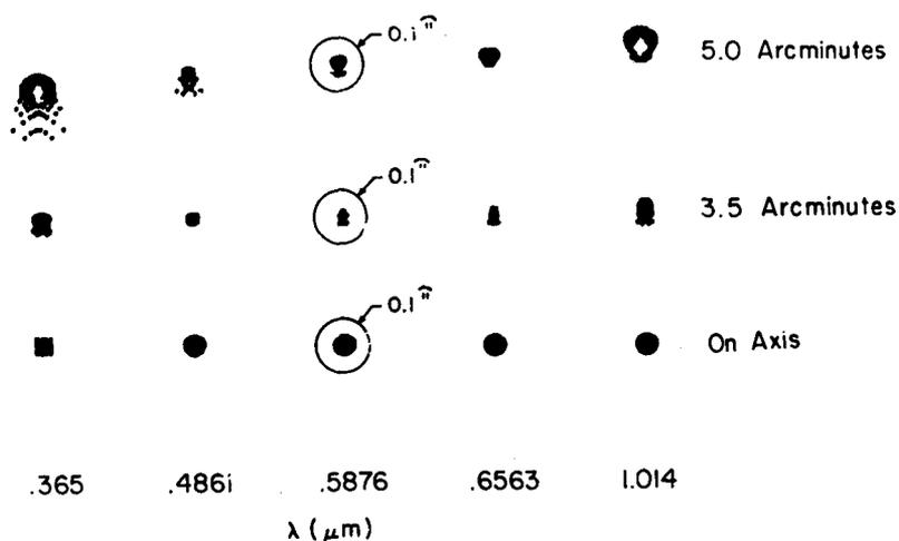
Figure 14. Spot diagrams for Figure 13.
