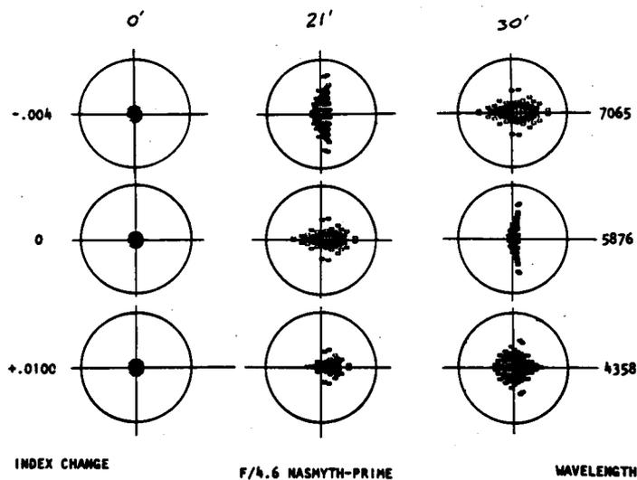
Figure 8. Spot diagrams for the f/4.6 camera of Fig. 7. The circle is 0.5 arcsec diameter.
