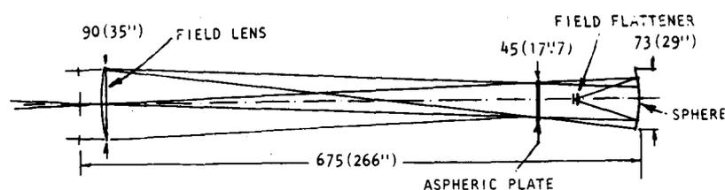
Figure 9. Meinel finite conjugate Schmidt focal reducer,  $f/1.5$ .
