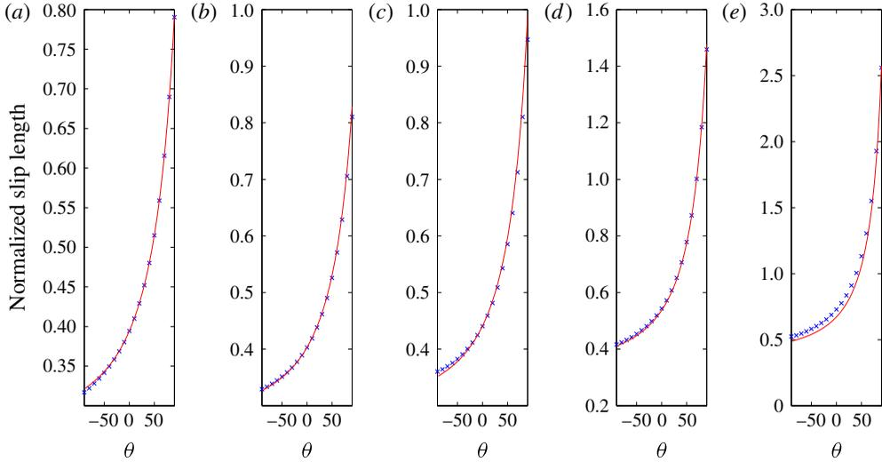
FIGURE 3. Normalized slip length, now based on the approximation  $\lambda_2$  in (4.13), as a function of  $\theta$  for  $c/l = 0.1$  (a),  $0.25$  (b),  $0.5$  (c),  $0.75$  (d) and  $0.9$  (e). Crosses show numerical data from Teo & Khoo (2010).
